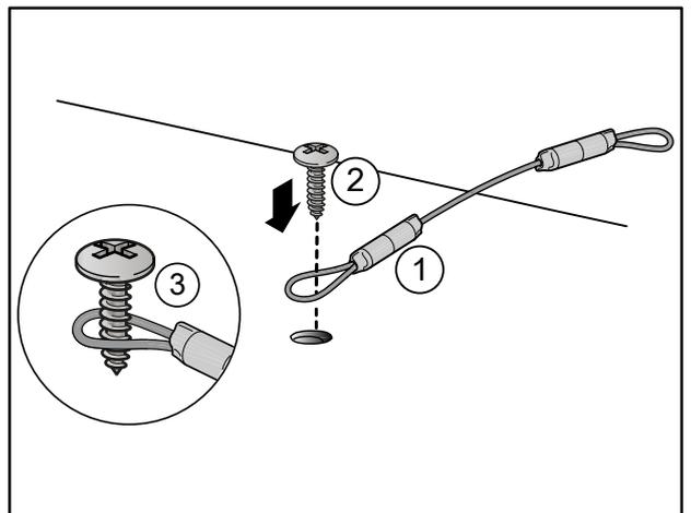
4. retighten the screw complete with the cable on the roof of the appliance;
