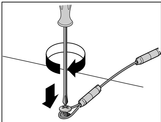
5. the cable must then be fixed to the wall with a plug, to permanently secure the appliance;
