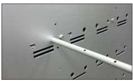
1. Insert the aluminum rod into the holes made in the center aluminum panel of the right compartment.
