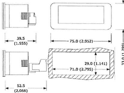
39.5 (1.555) is the depth with fixed screw connection terminal blocks; 52.5 (2.066) is the depth with removable screw connection terminal blocks.
