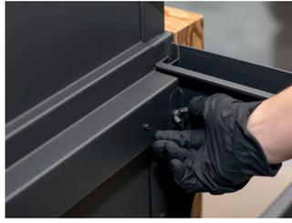
Remove the wing-screw on the right side, and remove the bracket that becomes free.
