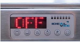
If the unit has been connected to the power supply, then “OFF” appears on the controller display
