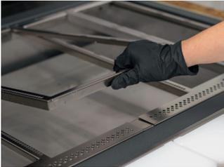
Depending on the configuration, remove the GN trays and their hook-in frames, and clean them separately. Clean the presentation areas with suitable cleaning agents according to Chapter 3.6.2.
