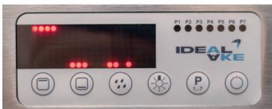
After being switched on, the controller always shows power level NEUTRAL in the display for all heat sources. The unit will not heat up. The light can be switched on and off. By pressing the buttons, the supporting heat 2, primary heat 3 and humidification 4 can be activated separately from each other with three levels each. The heating levels are shown visually on the controller display
