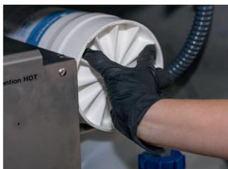
1. Switch the unit off at least 45 minutes before starting to replace the filter. The unit must be cooled down.
