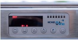
After switching on, the controller always shows the setting of the heating levels 2 and 3 on the controller display 1. The unit will not heat up. The light can be switched on and off 4.
