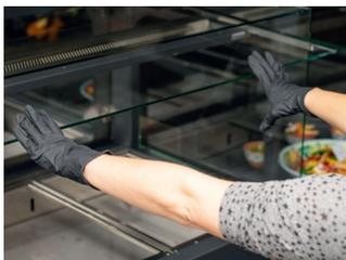
Lift the front glass and push it (guided by the built-in tracks) into the top end position as far as it will go.
