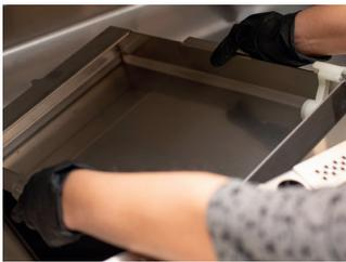
Remove the water bath using the handles provided. Carefully remove the float, and make sure that you do not twist it in the using the handles provided. The holder could break! Only clean the water bath after removal of the float. The float must be cleaned exclusively by hand. We recommend using a scale-removing cleaning agent that is suitable for stainless steel. Rinse all parts with clear water so that no residues remain.
