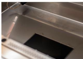
After the water bath has been removed (depending on the configuration), the interior of the bottom tray can be cleaned.
