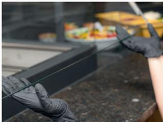
Grasp the the bottom of the front glass first with one hand and then with both hands safely in position.
