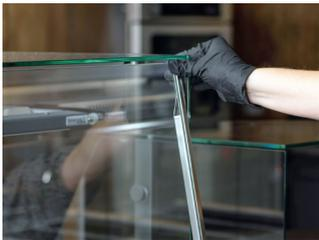
Press on one against one of the top corners of the front glass with one hand in order to swing out the bottom edge a few centimetres.
