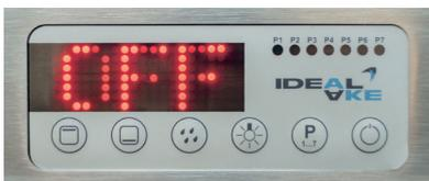
If the unit has been connected to the power supply, then "OFF" appears on the display
