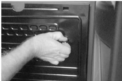
8. Dismantle the 5 evaporator clips. Press to release
