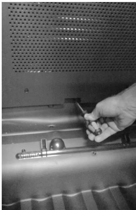
3. Dismantle 2 screws at the bottom ...
