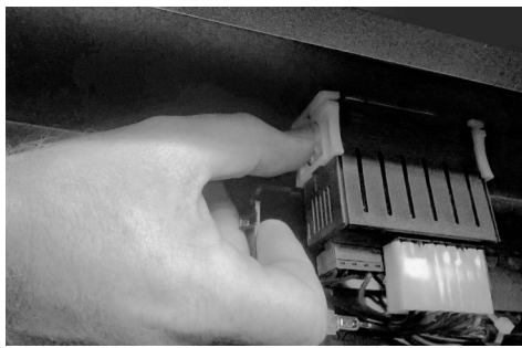
8. Push to release brackets for controller.
