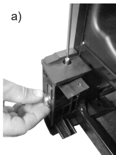
2. (a) Dismantle the lock pin before removing the lock, (b) Slide shoe is replaceable. a & b must be moved when reversing the door.
