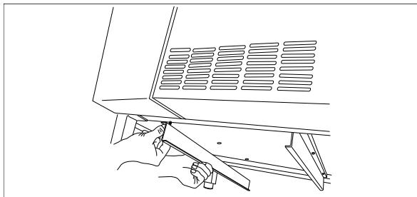
7. Take the tray located inside the compartment and slide it onto the support guides.
