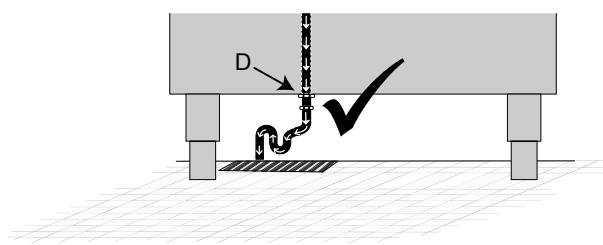
For 6GN 1/1 — 10GN 1/1 — 10GN 2/1 models , the drain diameter is 1½", therefore it is advisable to use a 1½" drain pipe or to a diameter 25mm hose.
