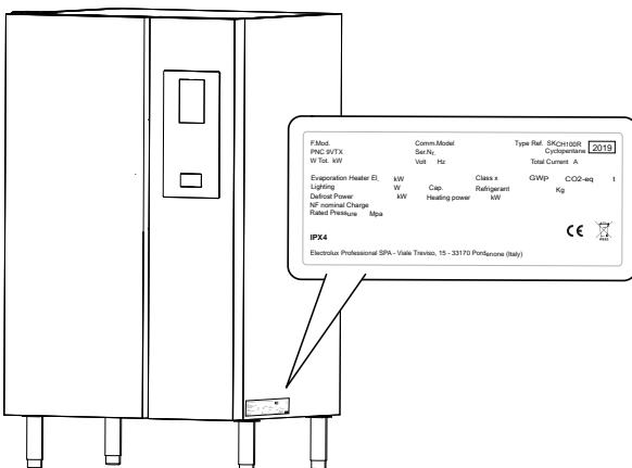
In **20GN 2/1** models the dataplate is located on the upper part of the left side of the appliance. The plate giving the appliance PNC code and serial number is located on the top of the appliance.
