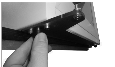
30. Remount and tighten the two front feet
