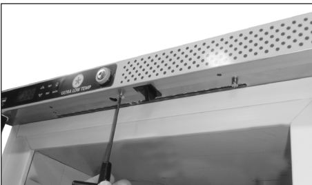
41. Remount the three screws upwards in the toppanel...
