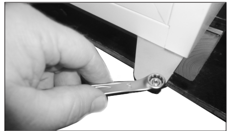
24. Remount and tighten pivot nut
