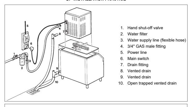
WARNING. This icemaker is not designed for outdoor installation and will not function in ambient temperatures below 10°C (50°F) or above 40°C (100°F). This icemaker will malfunction with water temperatures below 5 °C (40°F) or above 35 °C (90°F).
