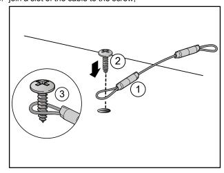
retighten the screw complete with the cable on the roof of the appliance;
