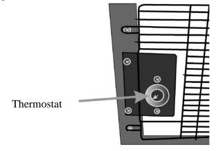
The thermostat can be adjusted with a scale of 1-6, which is equivalent to approximately 1-10°C Optimal setting will in most cases be 3-4.
